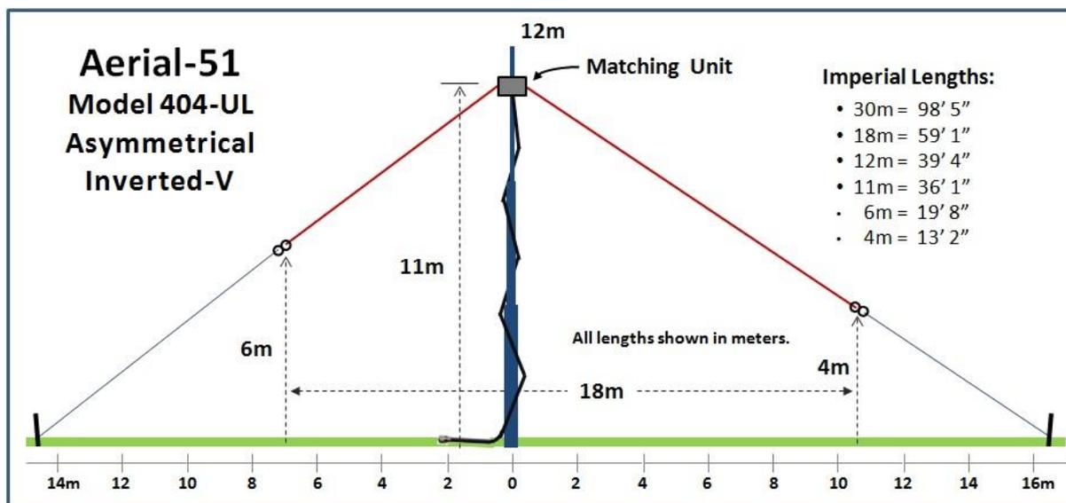
The Model 404-UL is a half wavelength long wire antenna on 40m. Though it uses a different feedpoint position, it works similar to a classical OCFD or dual-wire fed Windom. Whereas the original Windom design only covers even harmonic bands, the 404-UL was designed to also cover odd harmonic bands.
