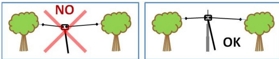
**DANGER:** When spanned between two trees as shown on the left, swaying of the trees in the wind may possibly break the wire of the antenna. Therefore, always support the antenna at its feedpoint, and then droop the wire legs slightly. There is no need to pull them tight. That only places unnecessary strain on the wire.
